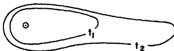
Figure 6. Propagation pattern of a simple channelized hydraulic fracture.
